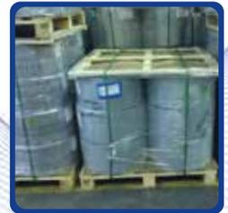
*PET Straps can be used in fully automatic pallet strapping machines during the packaging of products which require medium and high strength strapping. They can also be used by pneumatic strapping machines or battery powered strapping machines.*
